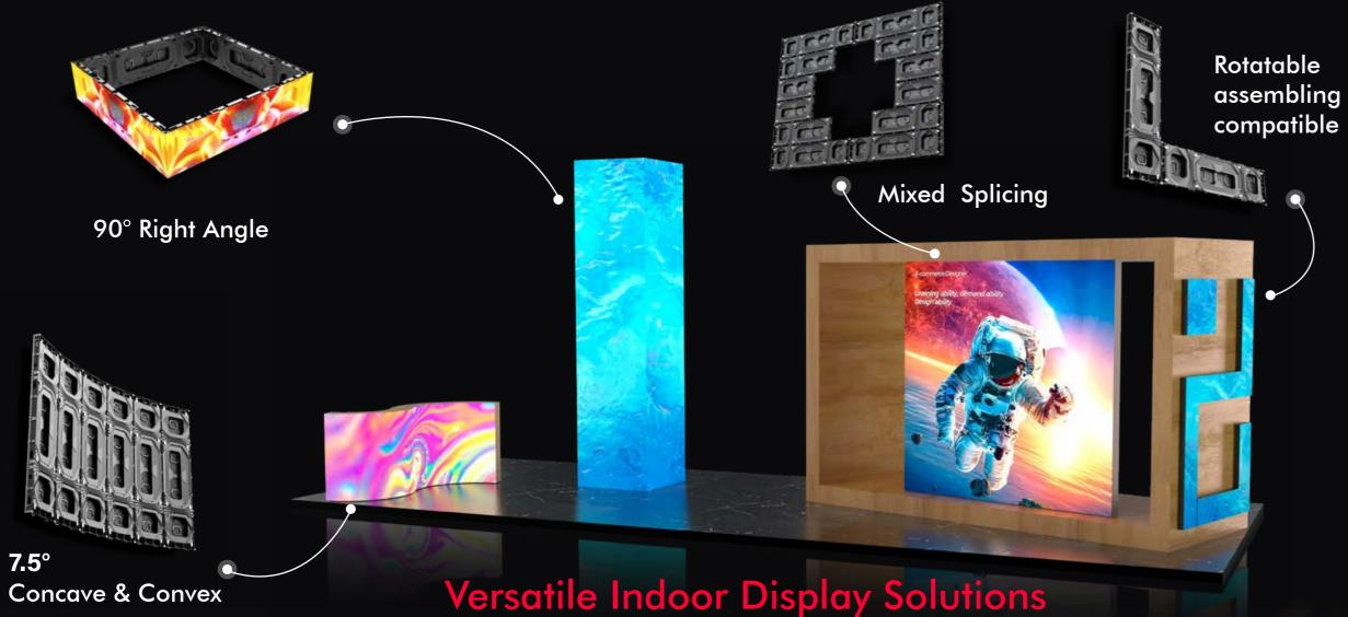
The Unity panel can be configured to create flat, curved, and column screens, making it a versatile solution that suits approximately 90% of indoor applications.
